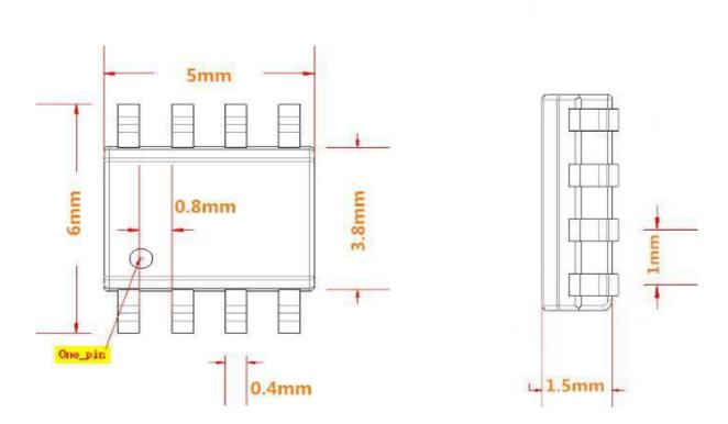
Unless otherwise prompted, all the sizes are marked as: (mm), tolerance: ±0.09mm
